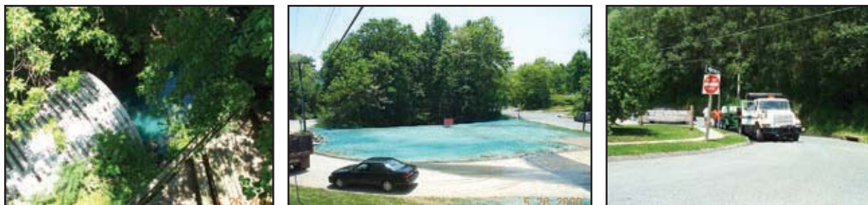
Figure 61: Symptom (left): Discoloration of stream; Diagnosis: Extra hydroseed leftover from an upstream application (middle) was dumped into a storm drain by municipal officials (right).
