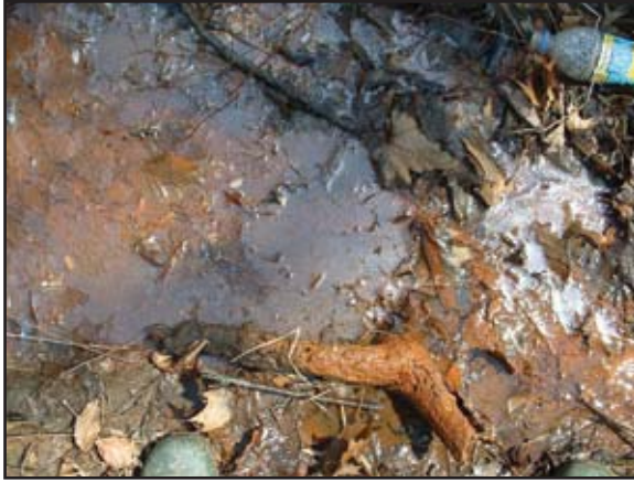
Figure 36: Synthetic versus Natural Sheen (a) Sheen from bacteria such as iron floc forms a sheet-like film that cracks if disturbed (b) Synthetic oil forms a swirling pattern
