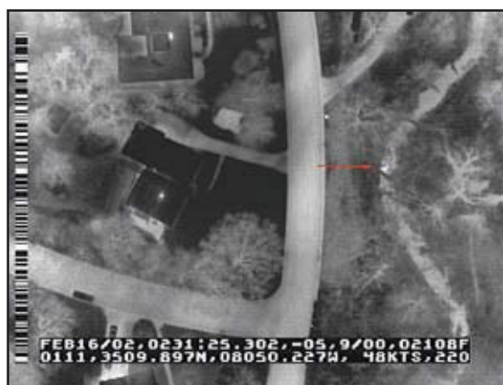
Figure 72: Aerial thermography showing sewage leak
