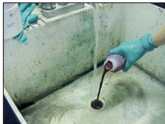
Figure 63: Dye Testing Plumbing (NEIWPCC, 2003)
